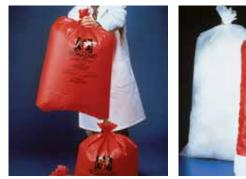
Heavy duty bags that can be loaded with used pipettes, Petri dishes, culture plates and membrane filters.
